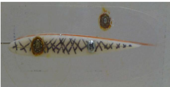
Figure – 6 Symmetric NACA 0011 Dimpled Airfoil
