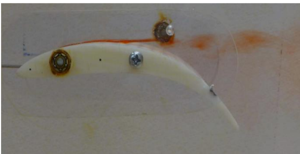
Figure – 7 Asymmetric NACA 16611 Dimpled Airfoil
