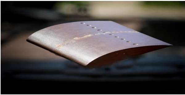
Figure 5 – Prototype of dimpled wing
