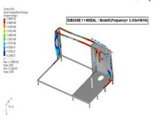
Modal analysis helps determine the modes of vibrations and these are the frequencies at which those modes are triggered.
