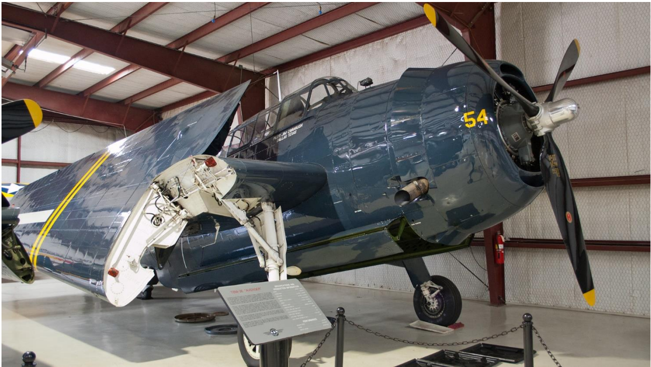
Fig. Grumman's TBM Avenger was one of the first aircraft incorporated with STO-Wing
