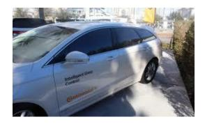
The latest technology used by an automobile manufacturer is the use of an electro chromic glass for sun protection. It is also known as intelligent glass control system, allows operator for automatic and manual tinting of car windows. User can adjust the transparency of glass according to the outside light conditions.
