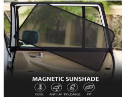
These are generally used by many people to keep the temperature inside the vehicle cooler under direct sun (usually in parking condition). Some sun shades use vacuum cups instead of magnet for easy sticking and removal. They are also helpful for UV ray protection. They are very useful for cars that are not having black films on them.
